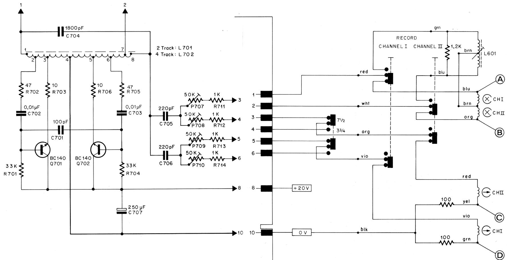
Position " Record - Stereo ", voltages measured against ground ( 0 V )
