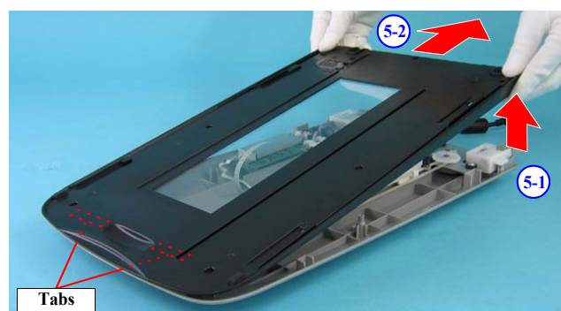
Figure 4-28. Removing TPU Lower Housing (2)
